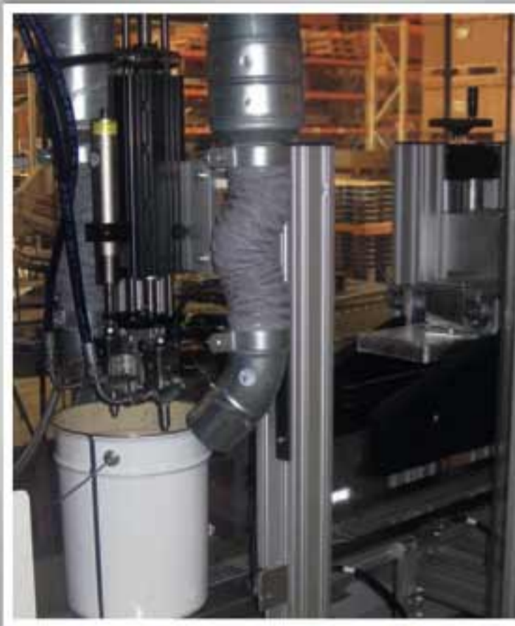
Latest development at Baltic is this system developed with Can Man for induction curing ear-weld repair spray coatings
