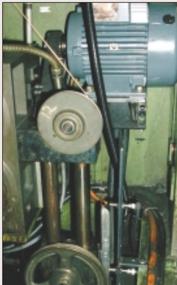
Wire speed on welders is automatically regulated using Sabatec's conversion kit
