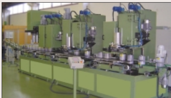
Quick format changes are a feature of Juan Capella's latest DRAC pail making system for sizes from three to seven litres
