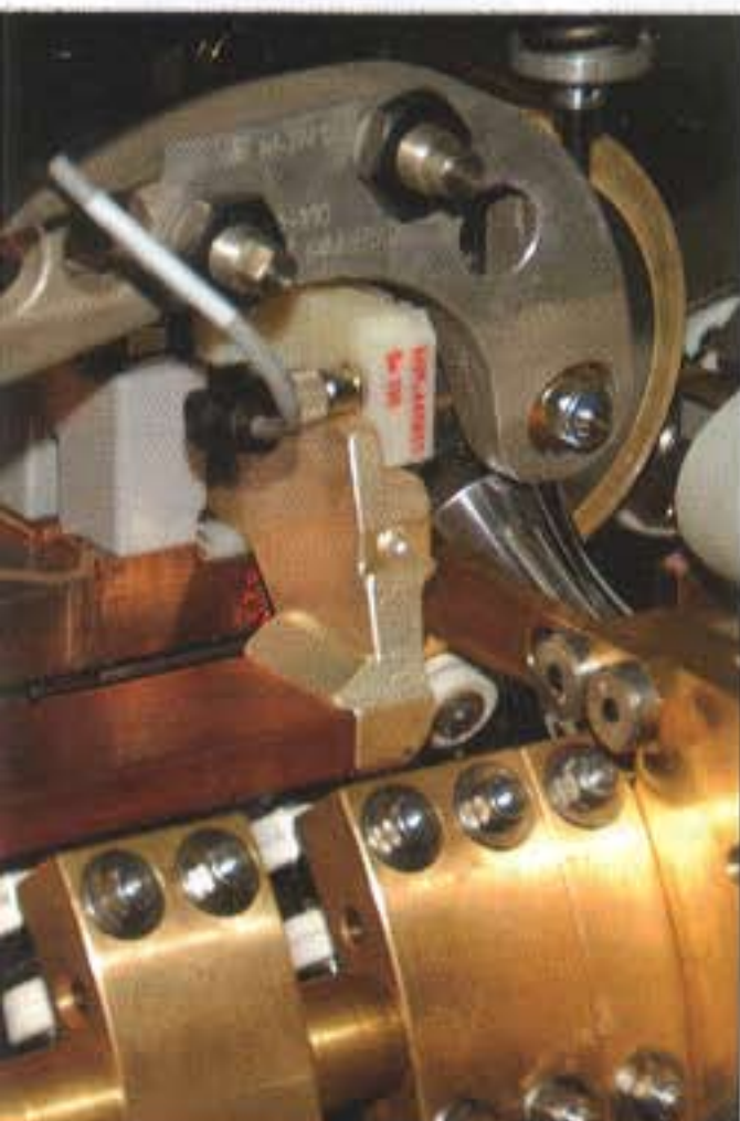
Top: Can Man's PowerCut slitter features pre-adjusted cutter shafts which may be removed by simply detaching the two brackets (inset) Above: Soudronic's continuous feeder offers automatic height changes and does not require operator assistance
