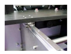
Use an oily cloth for this and clean the complete length of the rail or use a dry cloth to remove the dirt.
