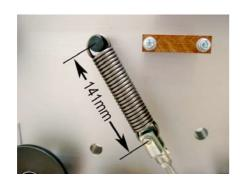
The setting for the distance: 141mm (measured without wire).
