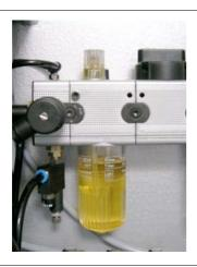
Check the amount of oil in the oil container. If necessary, fill the oil container up to the max. marking with "Tellus 27" from Shell or a similar oil.
