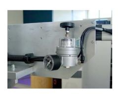
Check the pressure gauge of the wire loop of the type CM 16-300/400. Correct pressure setting: 2 bar
