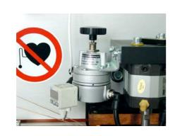
Check the welding pressure on the pressure gauge (manometer). The setting pressure should be between 2.5-3.0 bar (resp. 41-49 daN).
