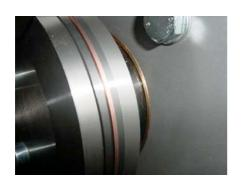
Clean the carbide steel surfaces of the wireprofiling unit. Check with your fingernail whether "tyre effects" are already present.
