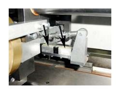
The two carriers of the linear guide. (Picture taken from the back of the machine)
