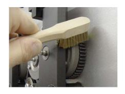
Use the small brush that was delivered with the machine and clean the transport wheels of the chopper. The transport wheels are the upper pair of wheels.
