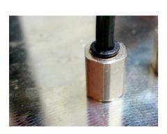
Check that there are no leaks anywhere in the air lines, and correct any leakages found.
