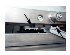
The two grease nipples, view and access from the front. Those should be lubricated with two shots of grease.
