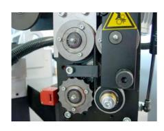
Check the gear wheels and the transport wheels of the chopper for wear or damage.
