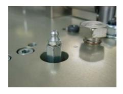
Apply 2-3 shots of grease to each grease nipple on the upper roller using the grease gun.
