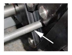
Apply some grease on the spindle of the canbody carrier (longitudinal travel direction).
