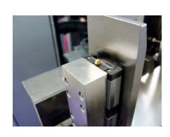
Inject grease from the supplied grease gun into the grease nipples of the two guide carriers, 2 shots are sufficient.
