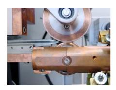
Check the wire grooves of the rollers and the corresponding edges of the same. Pay special attention, that the grooves are not crooked.
