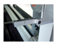
Check the fingers and the inner and outer transport belt for damages and wear.
