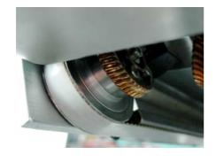
Also apply a little grease to the two worm gears (screw drives) that are accessible from the bottom.
