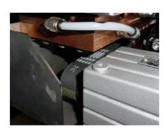
Check the belt tension of the pendulum head.
