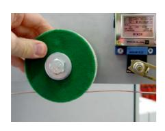
Turn the wheels of the wire cleaning through one quarter of a turn.
