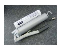
Make use of the supplied grease gun. The complete machine should be lubricated on a weekly basis.
