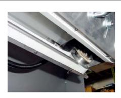
Check the belt for any visible external damage.
