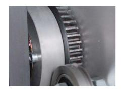
Apply a little grease to the flanks of the gears.
