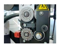
Check the position of the counter bearing at the chopping station and the condition of the cutting blade. Each individual blade should slightly touch the counter bearing and a relatively even sound should be audible when the wire chopper runs empty (i.e., without wire).
