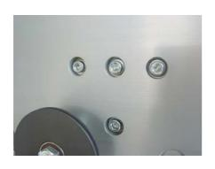
Check that all the screws are firmly seated, and in particular those on the welding circuit (transformer connections, roller head carriers, connecting rails, current leads).
