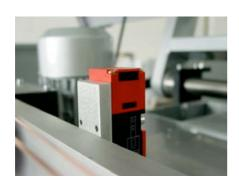
Check the function of safety switch (S 60.4) for the sliding door. The machine may not produce while the sliding door is open.
