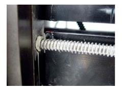
Apply a little grease to the spindle of the hand wheel adjustment.
