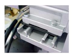
Undo the four M8 screws, and pull the motor unit to tighten the belt.
