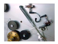
Check the wire tension in the wire loop. (only Type CM 16-200).
