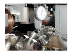
Check the radial clearance of the upper Diabolo rollers.
