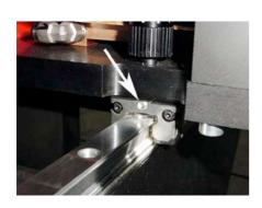
$2x \qquad \begin{array}{l} \text{Those two grease nipples on either linear} \\ \text{guide should be lubricated with two shots of} \\ \text{grease on a weekly basis.} \end{array}$
