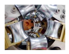
Clean the rollers of the pre-calibration and the Diabolo rollers.
