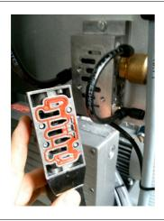
Take off the housing of the valve and clean the valve with compressed air, but only to a max. of 2 bar pressure! => Wear glasses!
