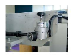
Check the pressure of the chopper gauge - the type CM 16-300/400. Correct pressure setting: 3 bar
