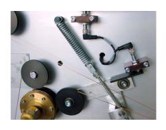
Alternative (only Type CM 16-200): Check the wire tension in the wire loop.
