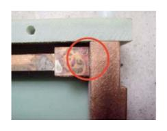
Check the screws, where they connect to the coil part.
