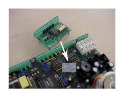
Install the extension PCB (printed circuit board) on the pacemaker main board.
