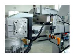
The eject station is a setup of various sensors and a "blower"/cylinder mounted to a conveyor belt within the range of max. of 250 canbodies from the welding station. It is activated through the weld-monitor and the frequency inverter.
