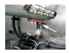
The height of the sensor can be adjusted here (arrow).
