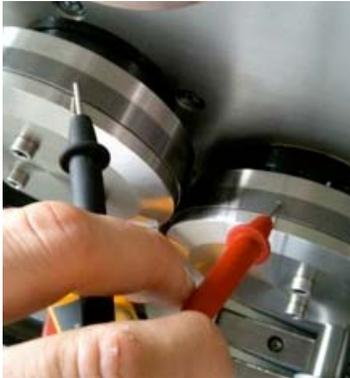
Measure between left and right carbide ring. The result on the Ohmmeter must be endless! This step is to ensure the proper insulation of both rear insulation rings around the taper roller bearings!
