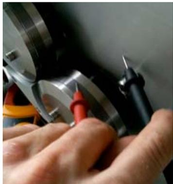
Measure the resistance between left carbide ring and main aluminum plate.
