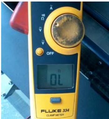
The picture shows the correct measuring result on the screen of the Ohmmeter for all three test points!
