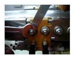
Set the precalibration roller pairs with a feeler gauge and a spanner 10 mm.
