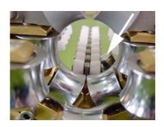
Check the welding sensor B6, there should be a clearance between 0.5 - 1.0 mm to the setting mandrel.
