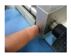
Both vertical alu-plates shall be even to the basic T-shaped basic plate. If not, undo on each vertical plate 2 x M10 from underneath, and move plates in a correct position.
