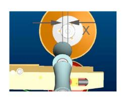
The center of the calibration crown (tooling) should be  $X=2-3\ \text{mm}$
