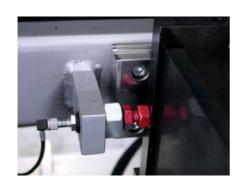
The screw with the lock nut has a red seal and must not be changed. This is used to fix the position on the longitudinal axis of the tool carrier with regard to the welding centre.
