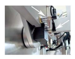
The sensors B1 and B2, which are mounted to main machine plate, need to be readjusted.
