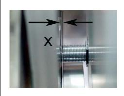
The reason, why the wire is still running is, that a distance "x" in the picture is too big. Therefore reduce the clearance for both sensors B1 and B2 too a minimum of 0.1 mm.
