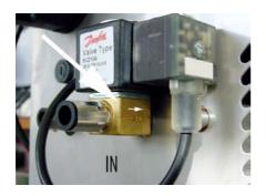
Check the correct water flow direction.
