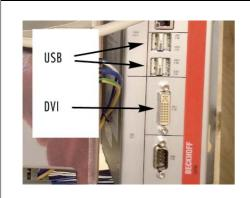
In case of a trouble shooting, you are able to connect a disposable keyboard and monitor to the PC, in order to observe the booting process, that appears to be faulty or out of order.
