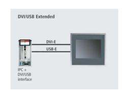
The digital visual interface (DVI), transfers the PC image digitally to the display. The universal serial bus (USB) enables connection of input devices and drives to the PC.
