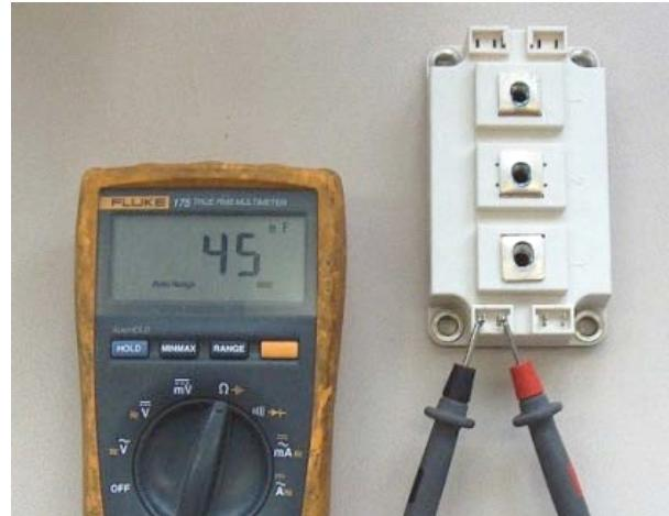
You can also check the switch of the IGBT. For this test you must start the system and bring it to the state "Stand by". Measure the resistor of the switch with a diode test controller as following:
