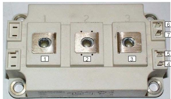
Further, you can also measure the input capacitance between gate and emitter.
