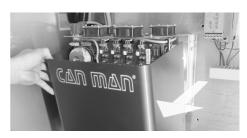
3. Switch machine power ON
