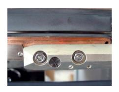
Undo the two M6 nuts only from the front side, not from the backside, in order to keep the position.
