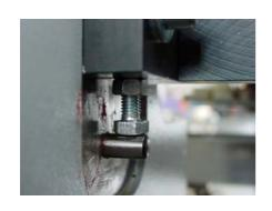
Then use the M10 screw underneath to make the necessary adjustments.
