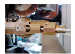
The lower welding roll need to be replaced by the "dummy roll", for this, undo the two screws that clamp the roller head axis.
