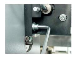
To make the necessary adjustments you need to loosen the two M10 screws of the fixture.
