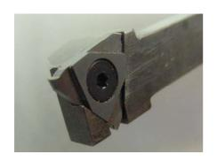
Original Can Man redressing tool. It was designed specifically for the exact redressing of the wire profile in the electrode wheel heads.
