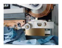
Take the outside welding roll holder off, be aware that some cooling water will come out from the cooling circuit of the lower welding roll.
