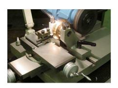
To ensure that the maintenance of the electrode wheel heads is carried out exactly and efficiently manner, we urgently recommend the procurement of a so-called welding roller redressing unit, type CM 91.
