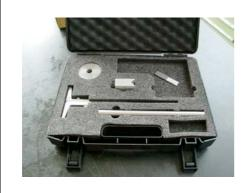
A complete set of gauges is supplied to enable the important settings of the welding geometry to be made in a proper manner.
