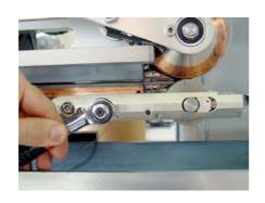
Mount the "dummy roll" together with the shaft into the welding roll holder.
