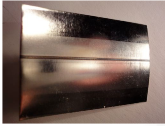
Back side showing tin re-flow
