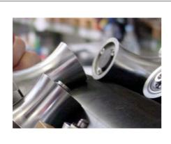
Bearings of diabolo rolls are worn out (therefore tooling is too tight in order to keep the overlap in the middle of the canbody).
