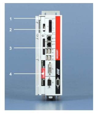
Opening the front flap (1) allows access to the battery (2), the CF-Card/ CFast-Card (3) and the hard disk (4) (optional).
