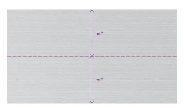
\* The scoring line must always be exactly in the middle of the cylinder height. Both, the deviation of the score line (in height) as well as the offset at the welded seam (at the side), must be within  $\pm$  0.1 mm. Larger deviations may result in problems because the score line is no longer flush with the parter.
